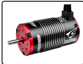
C-54055 Electric Motor - Kuron 825 - 4-Pole - 2050 KV - Brushless - Sensorless
